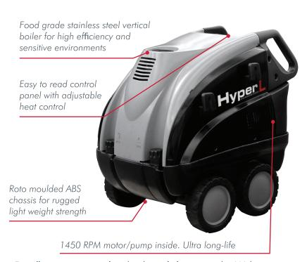
For all your commercial and industrial cleaning tasks. With maximum reliability, the best technology and components including a stainless steel boiler coil and a low speed 1450 RPM linear pump unit with high pressure detergent application, these single phase machines work continuously at top performance! 140°C destroys grease and food grime on transport and farm equipment. Complete with heavy duty gun, nozzle, lance and 10m wire braided high pressure hose.
